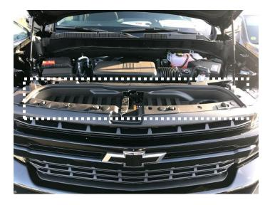
2. The cover is held in place with push style plastic fasteners. To release them, pry up the head with a standard screwdriver in the grooved portion pictured below. Then pry the entire fastener out of the cover and set aside. Remove all until the cover is free.
